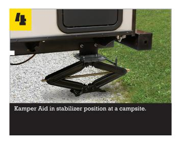
Travel trailers are built low to the ground for stability and aerodynamics, but when parked they require stabilizer jacks for leveling which can scrape and damage the jack and trailer when traveling in low ground clearance situations. With the Kamper Aid adapter, the stabilizer jack easily swings up and out of the way providing increased ground clearance, less costly jack replacements, less damage to your trailer, and a smoother, more enjoyable travel experience.
